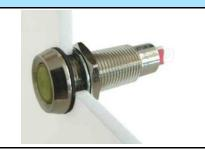
Ø8.1mm Mounting Bright Nickel Plated Brass Housing Smoked Lens - Good On/Off Ratio High Intensity LED Colours Internal Resistor - Voltage Options Sealed to IP67 - Weatherproof Durable to Shock and Vibration
